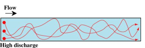
**Turbulent Flow**: every fluid molecule followed very complex path that led to a mixing of the dye.
