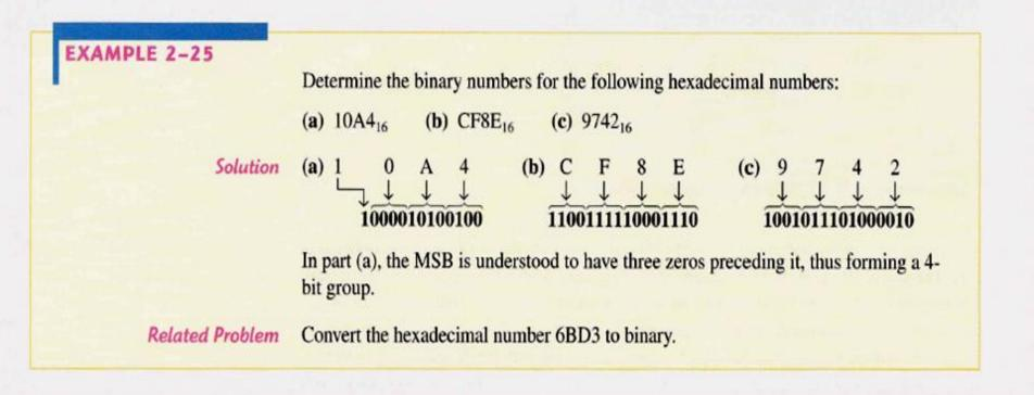
It should be clear that it is much easier to deal with a hexadecimal number than with the equivalent binary number. Since conversion is so easy, the hexadecimal system is widely used for representing binary numbers in programming, printouts, and displays.
