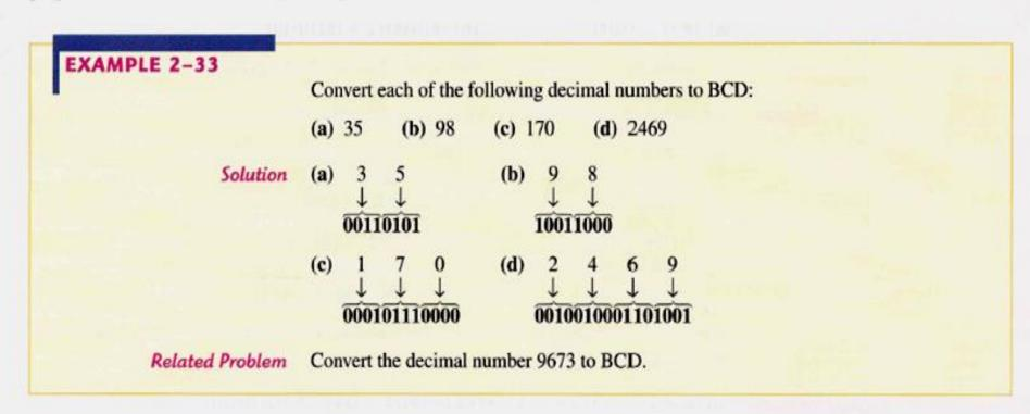
It is equally easy to determine a decimal number from a BCD number. Start at the rightmost bit and break the code into groups of four bits. Then write the decimal digit represented by each 4-bit group.
