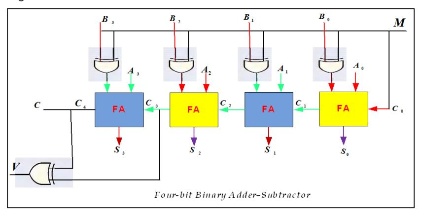
The mode input M controls the operation as the following:
