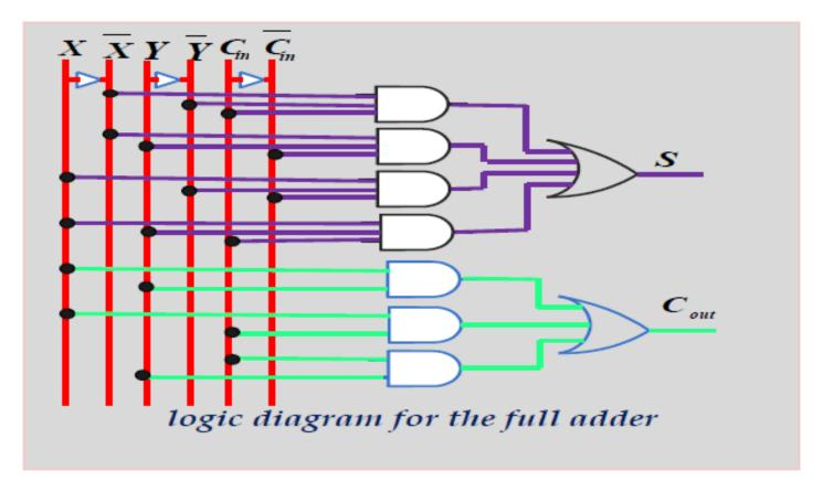
➤ It can also be implemented using two half adders and one OR gate (using XOR gates).
