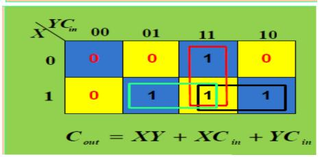
$$\begin{cases} S = \overline{X} \, \overline{Y} C_{in} + \overline{X} \overline{Y} \overline{C_{in}} + \overline{X} \overline{Y} \, \overline{C_{in}} + \overline{X} \overline{Y} \, \overline{C_{in}} \\ C_{out} = \overline{X} \, \overline{Y} + \overline{X} \overline{C_{in}} + \overline{Y} \overline{C_{in}} \end{cases}$$
